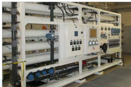
Figure 4: Example of Prefabricated Skids
