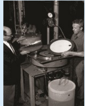
Professor Sidney Loeb and engineer Ed Selover remove newly manufactured reverse osmosis membrane from plate-and-frame production unit circa 1960.
