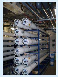
Separation of sugars such as dextrose and maltose from fibrous and undesirable proteins while purifying the mixture can be done with membranes. Clarification of the process stream after saccharification has been done in different facilities. Gelatin, egg whites, soy protein and other natural products can be improved using microfiltration and ultrafiltration.
