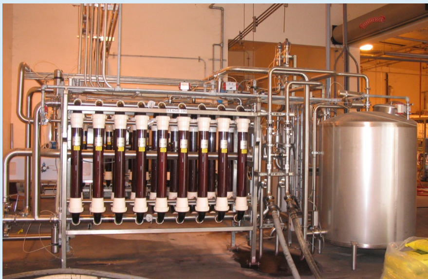
“Wine Processing System, photograph courtesy of KOCH Membrane Systems”
