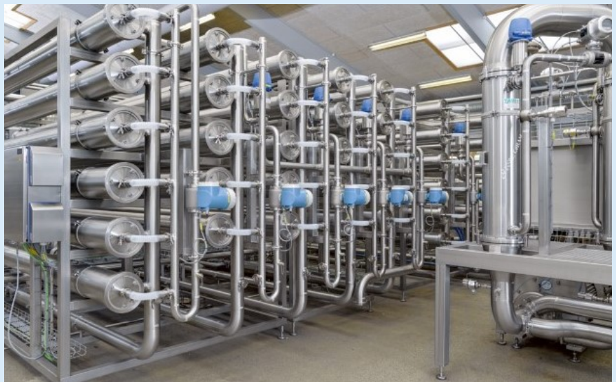
"Ceramic Microfiltration and Reverse Osmosis system for skim milk processing, photograph courtesy GEA Processing Engineering, Inc."
