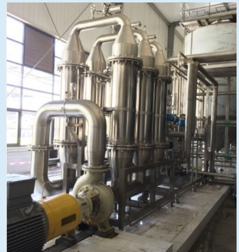
"Ceramic membrane system for beer processing, photograph courtesy GEA Processing Engineering, Inc."
